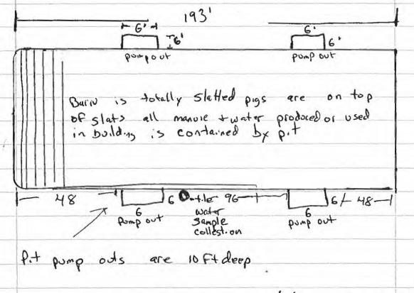
Manure is pumped out of 6x6 pump outs by either manure wagon with bx 6 inch manure pump attached to a drag line pumping system to incorporate manure into sol for use as Fortileer For crops
